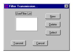
The user filters in the SMIQ are displayed in the 'UserFilter List'. A maximum of 4 user filers can be stored in SMIQ. To create a new UserFilter:
